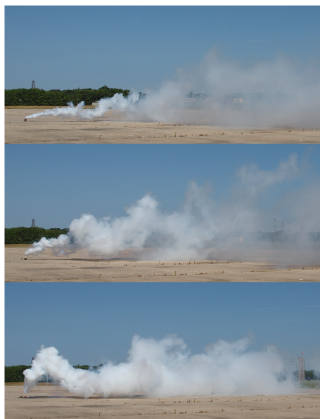
Figure 3. Smoke screens produced by end-burning BC smoke grenades, midburn: type 1 (top), type 2 (middle), and type 3 (bottom).
