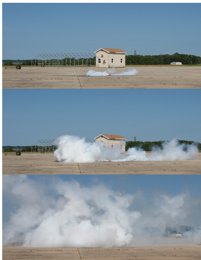
Figure 4. Time sequence for a core-burning BC smoke grenade containing the type 3 composition. Images show smoke screen formation at 0.4 s (top), 2.8 s (middle), and 8.0 s (bottom). Total grenade burning time was 3.5 s.
